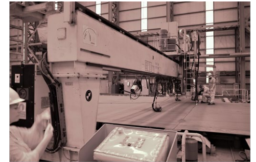
Above: Automated SAW gantry system on a panel line.
